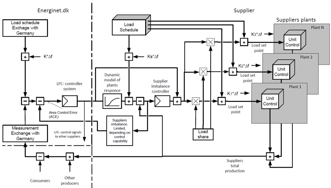
Figure 7 Principle for the design of the system in DK1 where the BRP has a Supplier imbalance controller.
