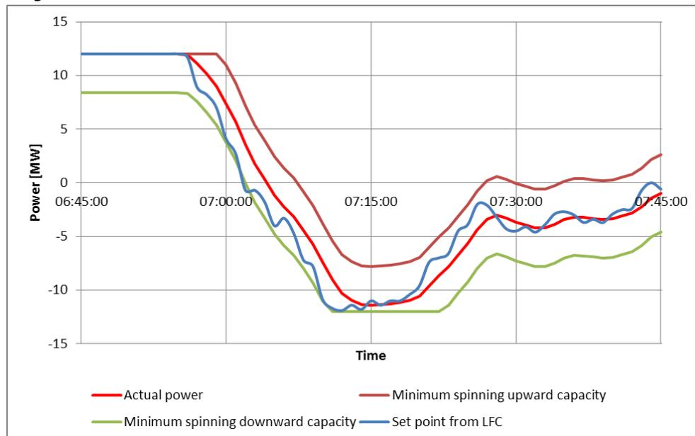
Figure 4 Example of a schedule for activation of FRR-A in DK2 from a capacity of +/- 12 MW.
