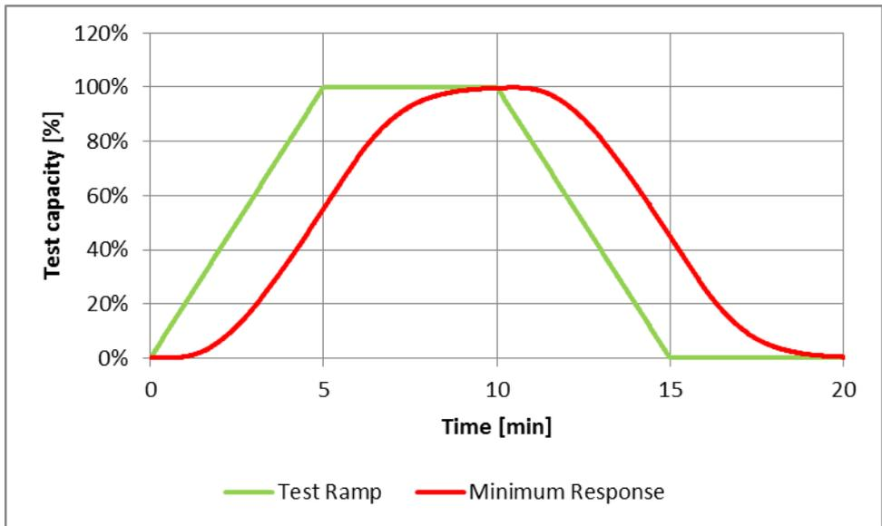
Figure 2 Example of requirements when the unit/portfolio is tested against a ramp in DK2, where the response between 20% and 80% shall be at maximum 135 seconds delayed from Test Ramp
