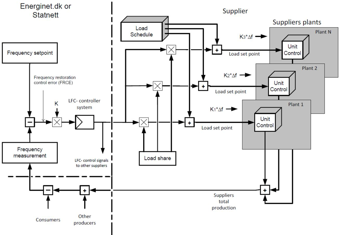
Figure 6 Principle for the design of the system in DK1 where the BRP has no Supplier imbalance controller.
