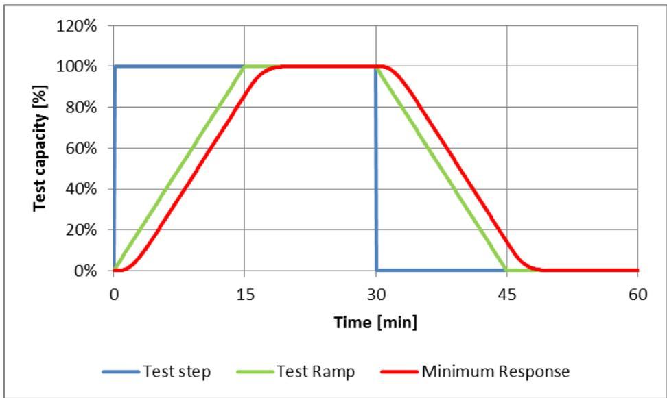
Figure 3 Example of required response when the unit/portfolio is tested against a step **or** a ramp set-point change in DK1, where the response between 20% and 80% shall be at maximum 135 seconds delayed from Test Ramp values. 85% of full activation has to be reached within 15 min
