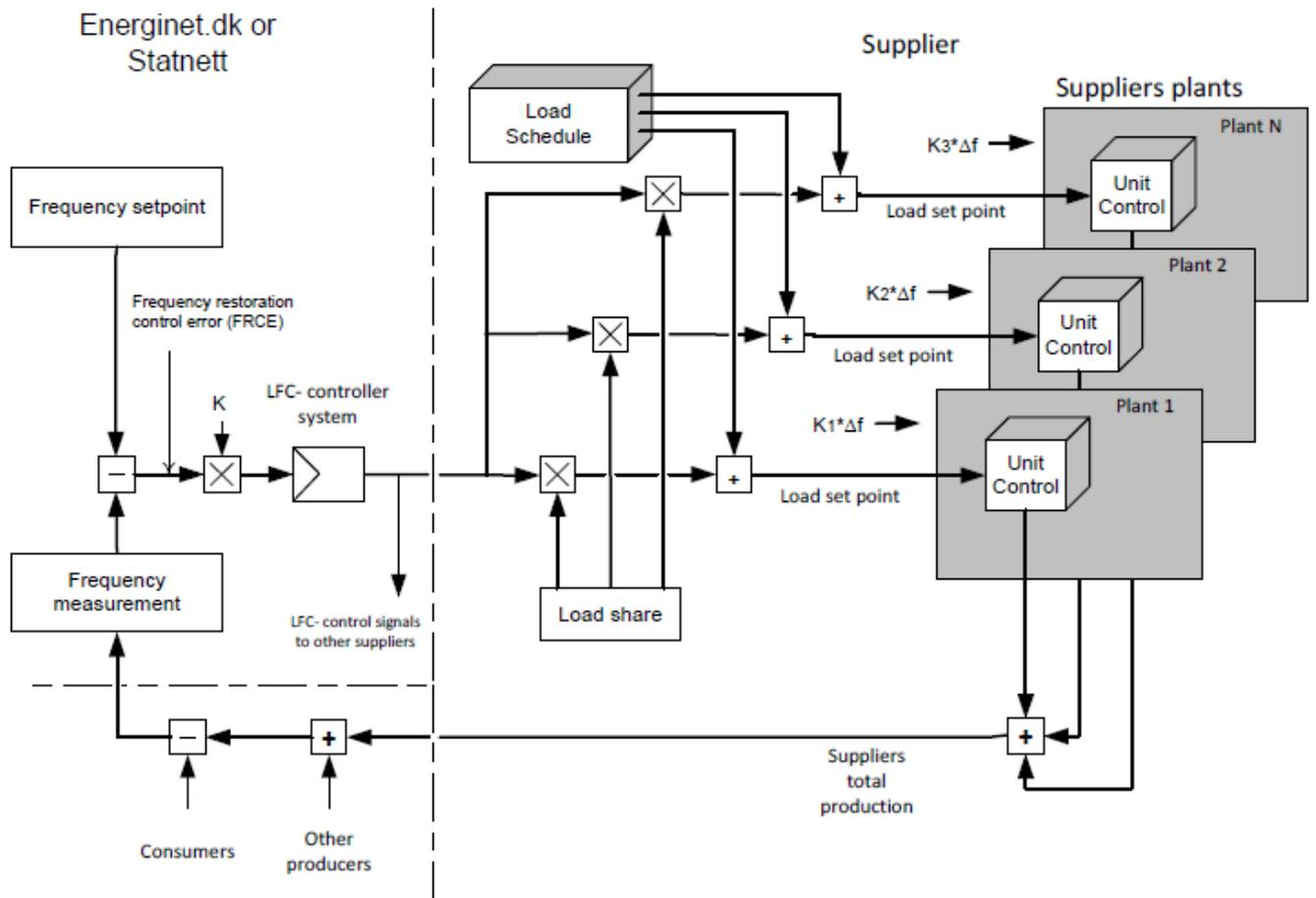
Figure 5 Principle for the design of the system in DK2 where the BRP has no Supplier imbalance controller.
