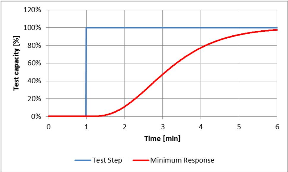
Figure 1 Example of minimum response when the unit/portfolio is tested against a step set-point change in DK2, where 90% of full activation has to be reached within 5 min
