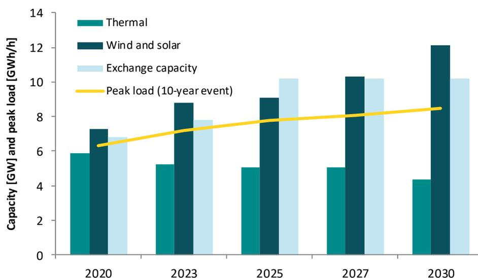
Figure 4 Electricity generation and exchange capacities as well as maximum electricity consumption in case of a 10-year incident for Denmark as stated in the *Analysis assumptions for Energinet 2018* report.
