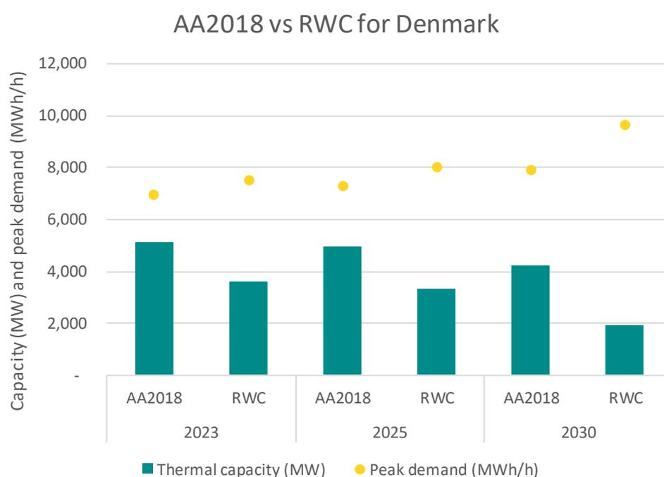
Figure 5 Thermal electricity capacity and maximum electricity consumption for Denmark based on Analysis assumptions for Energinet 2018 and the RWC scenario.
