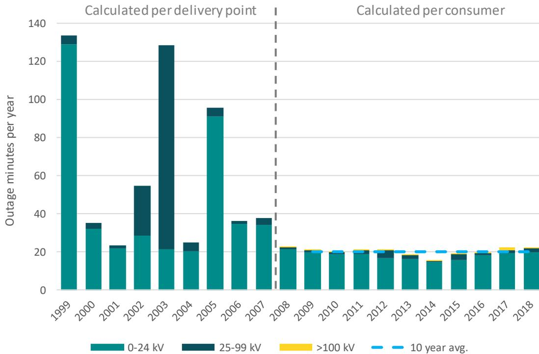
Figure 2 Outage statistics for Denmark, 1999-2018. Calculations for 1999-2007 are per delivery point (fictitious point in the 10 kV grid), and calculations for 2008-2018 are per electricity consumer. Source: Grid operators' fault and outage statistics (Elselskabernes Fejl- og Afbrudsstatistik (ELFAS)), Danish Energy.
