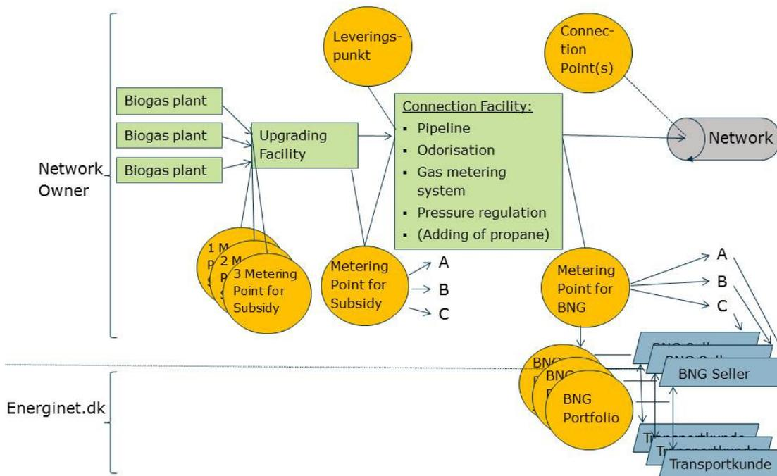
In so far as more than one Biogas Plant is served by the Upgrading Facility and the Network Owner is responsible for the meterings, the Network Owner meters, at the Metering Point for Biogas, the injection of Biogas from the Biogas Plant to the Upgrading Facility. The Network Owner submits metering data from the point to the Biogas Producer, the Upgrading Facility Owner and Energinet.dk.
