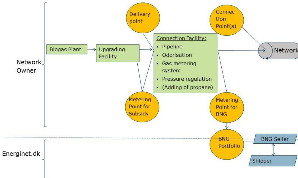
The Biogas Plant is the plant producing Biogas. The Biogas Producer is responsible for the Biogas Plant.
