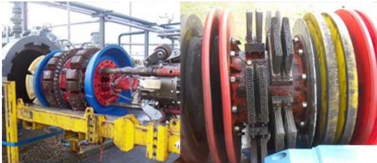
Inserting an intelligent pig in a gas pipeline (left) and a cleaning pig with a gauge plate (right).
