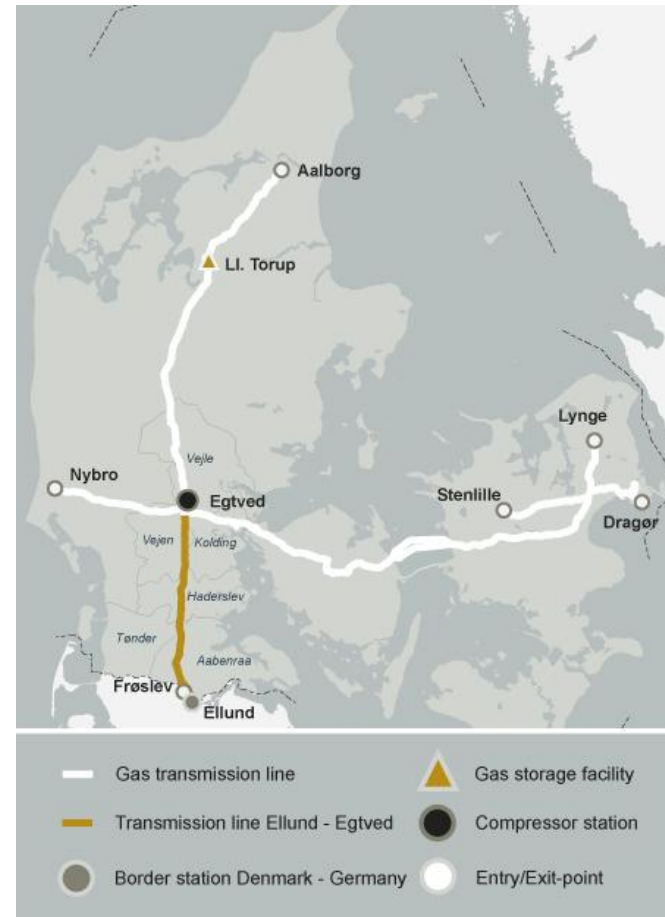
The Danish main transmission system for natural gas with a compressor station in Egtved and an Ellund-Egtved looping.
