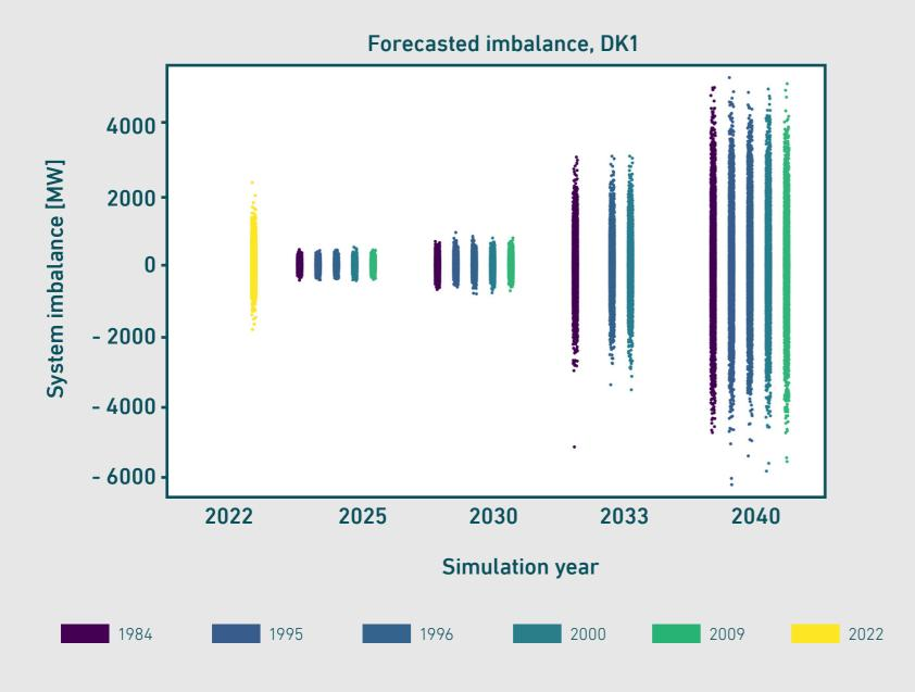
The two graphs show the simulated hourly imbalances on the y-axis with the respective years on the x-axis, differentiated by various climate years represented by different colours. These simulations incorporate forecast errors derived from a Monte Carlo simulation.
