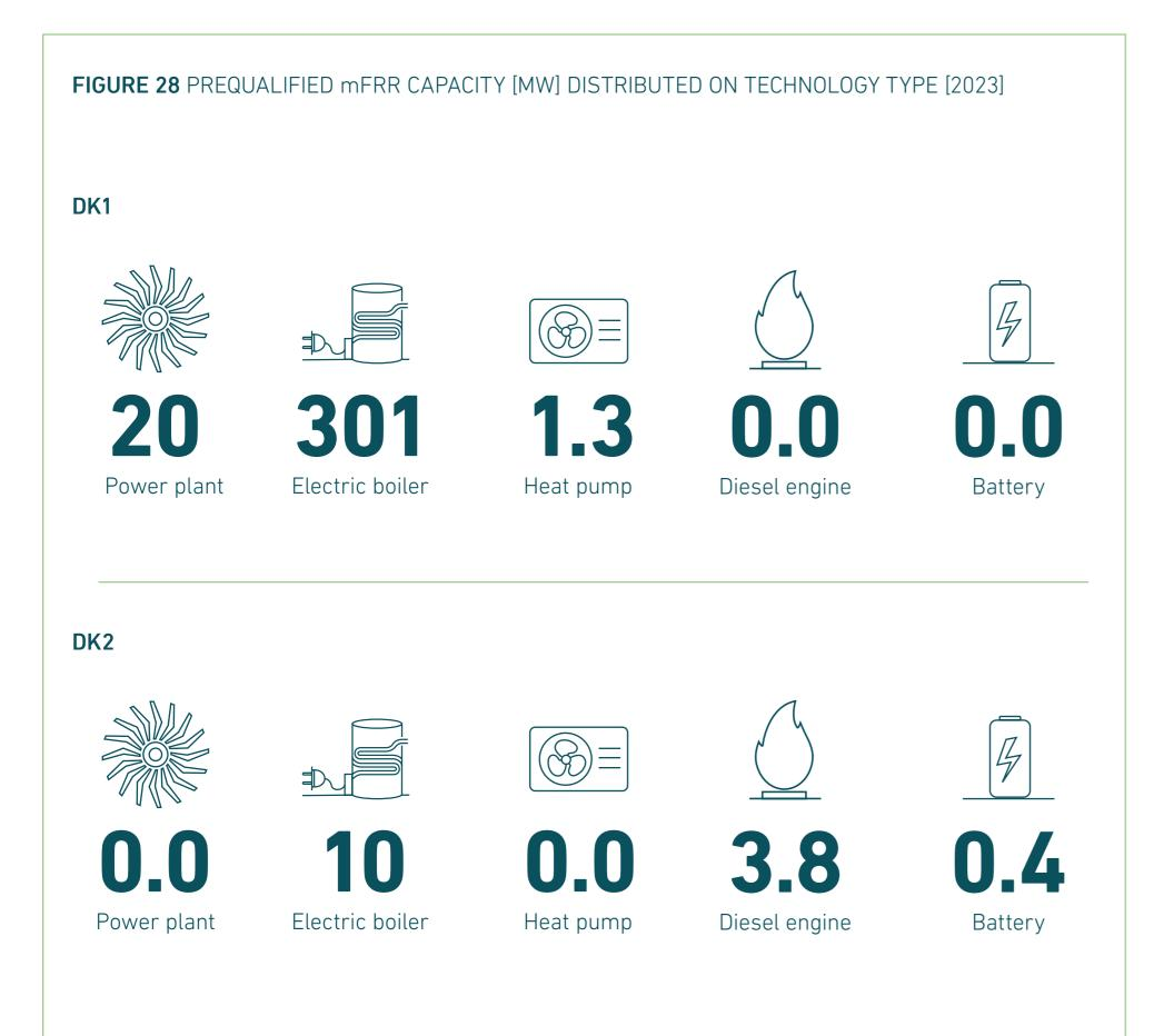
In 2023, 322.3 MW new facilities have been prequalified to deliver mFRR in DK1, and 14.2 MW have been prequalified to deliver mFRR in DK2. Figure 28 shows the share of different technologies. In both DK1 and DK2, electric boilers have contributed the largest share of mFRR prequalified units.
