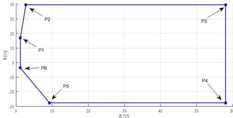
Figure 3 Example of grid impedance polygon descriptive of grid impedance at the electricity generation facility's Point of Connection.
