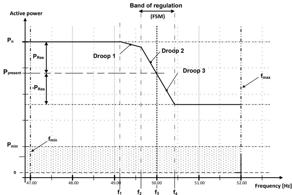
Figure 11 General frequency control principle for a plant.
