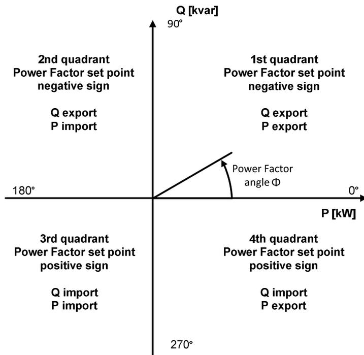
Figure 1 Definition of signs for active and reactive power and Power Factor set points [ref. 16 and 17].
