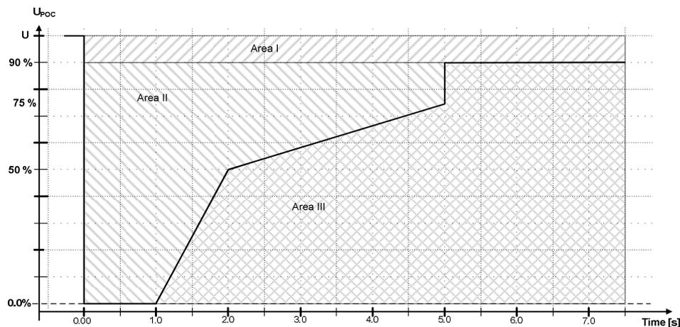
Figure 6 Tolerance requirement for single-phase voltage dips for plants in category B and C.
