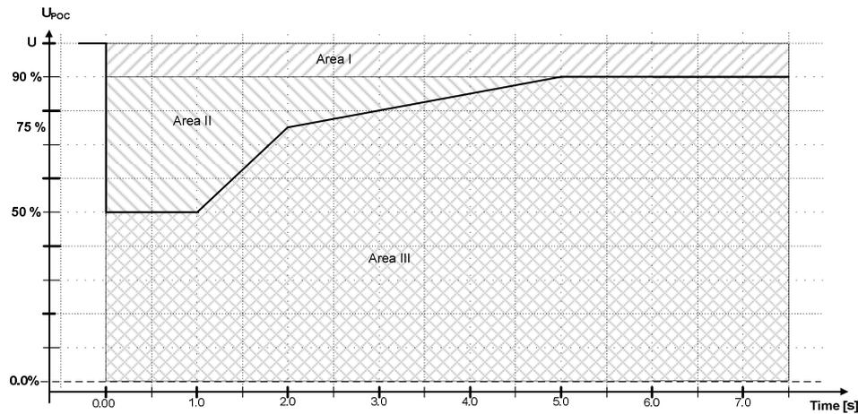
Figure 5 Tolerance requirements for three-phase voltage dips for plants in category B and C.
