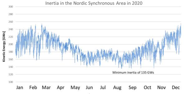
*Figure 3. Estimated kinetic energy values (pre-disturbance values<sup>4</sup>) from the online kinetic energy estimation tool for the Nordic synchronous system in the year 2020.*
