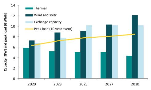
Figure 4 Electricity generation and exchange capacities as well as maximum electricity consumption in case of a 10year incident for Denmark as stated in the Analysis assumptions for Energinet 2018 report.
